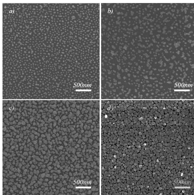
**Figure 1.** SEM images of bare AuNPs assembled onto APTES-modified electrodes (a), after 2 h of treatment in the solution containing 150 mM glucose and 300  $\mu\text{M}$  HAuCl<sub>4</sub> for 1  $\mu\text{M}$  probe **1** (b), the obtained dsDNA of 1  $\mu\text{M}$  probe **1** hybridized with 1  $\mu\text{M}$  target DNA (c), and the ultrapure water (d).
