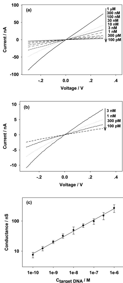
**Figure 4.** (a) Typical  $I$ - $V$  response curves for different target DNA concentrations from 100 pM to 1  $\mu$ M. (b)  $I$ - $V$  response curves for target DNA concentrations from 100 pM to 3 nM. (c) Calibration curves of the logarithm of conductance vs the logarithm of target DNA concentration for this electrical biosensor. Other reaction conditions are as for Figure 2. Error bars show the standard deviation of five experiments.
