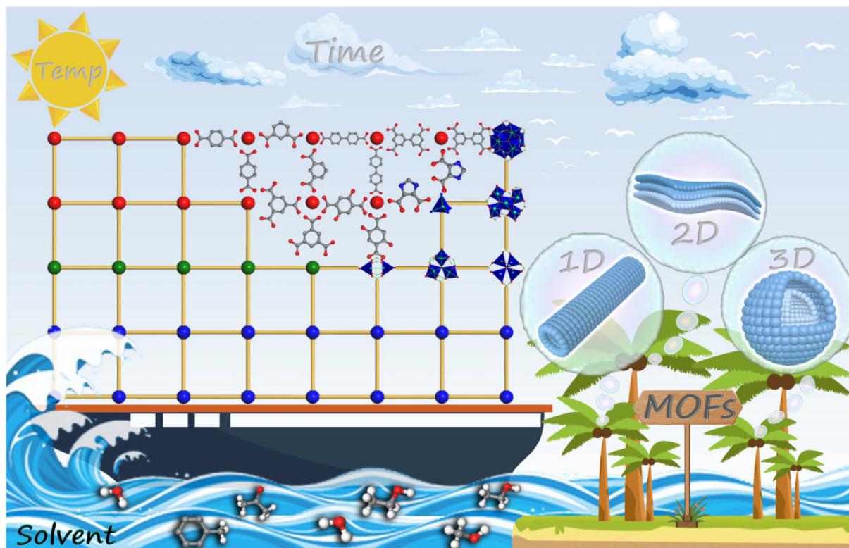
Scheme 1. Illustration for the construction elements of structure-induced MOFs. Here, the sun, clouds, ship, and sea represent the temperature, time, reaction vessel, and solvent, respectively, which are the basic conditions for the synthesis of MOFs. Finally, the crystals with 1D tubular, 2D sheet and 3D spherical morphologies can be synthesized in a controlled manner by changing various metal ions, organic ligands, and synthesis conditions.
