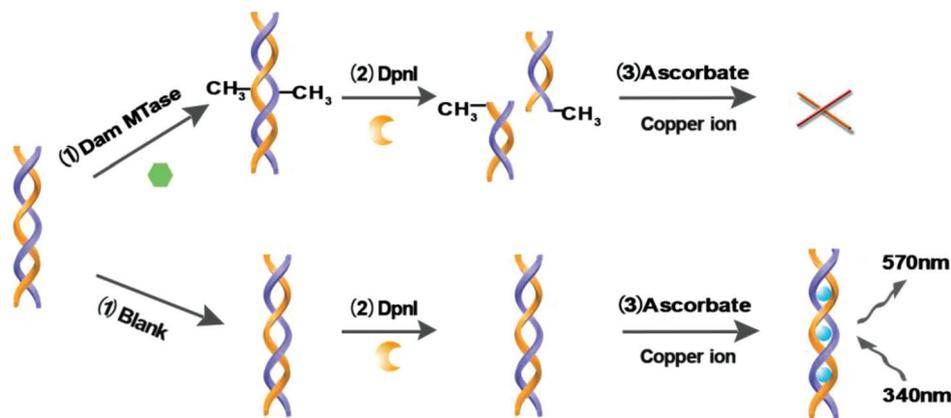
Fig. 1 Schematic diagram of the developed label-free fluorescence strategy for Dam MTase activity assay based on dsDNA-templated CuNPs coupled with an endonuclease-assisted signal transduction system.
