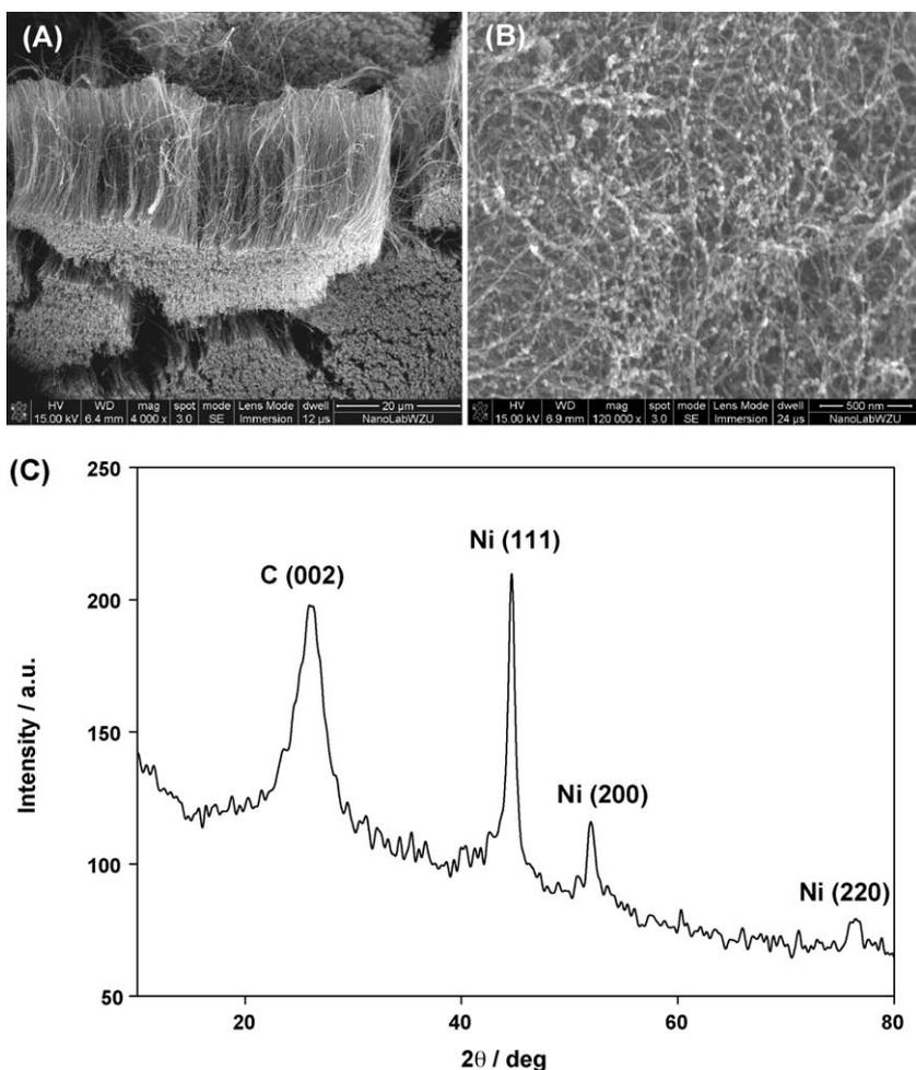
Fig. 1. Typical SEM images of SMWNTs (A), and NiNPs/SMWNTs nanohybrids (B) and XRD pattern of the NiNPs/SMWNTs nanohybrids (C).
