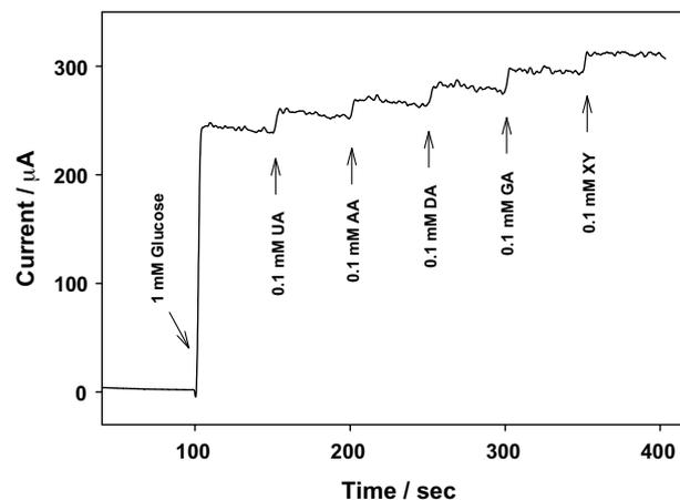
**Fig. 5.** Amperometric response of the NiNPs/SMWNTs modified electrodes with successive addition of 1.0 mM glucose, 0.1 mM UA, 0.1 mM AA, 0.1 mM DA, 0.1 mM GA, and 0.1 mM XY in 0.1 M NaOH solution at +0.4 V.
