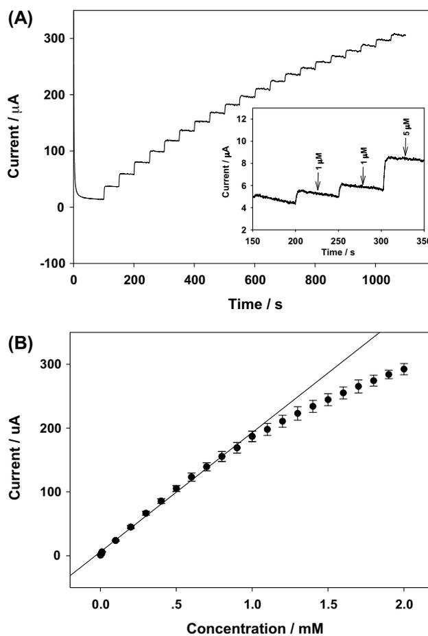
**Fig. 4.** Amperometric responses of the NiNPs/SMWNTs modified electrodes to successive addition of 100  $\mu\text{M}$  glucose in 0.1 M NaOH at +0.4 V (amperometric response of NiNPs/SMWNTs modified electrodes with the addition of 1  $\mu\text{M}$ , 5  $\mu\text{M}$ , 10  $\mu\text{M}$ ) (inset) (A) and its corresponding calibration plot (B).
