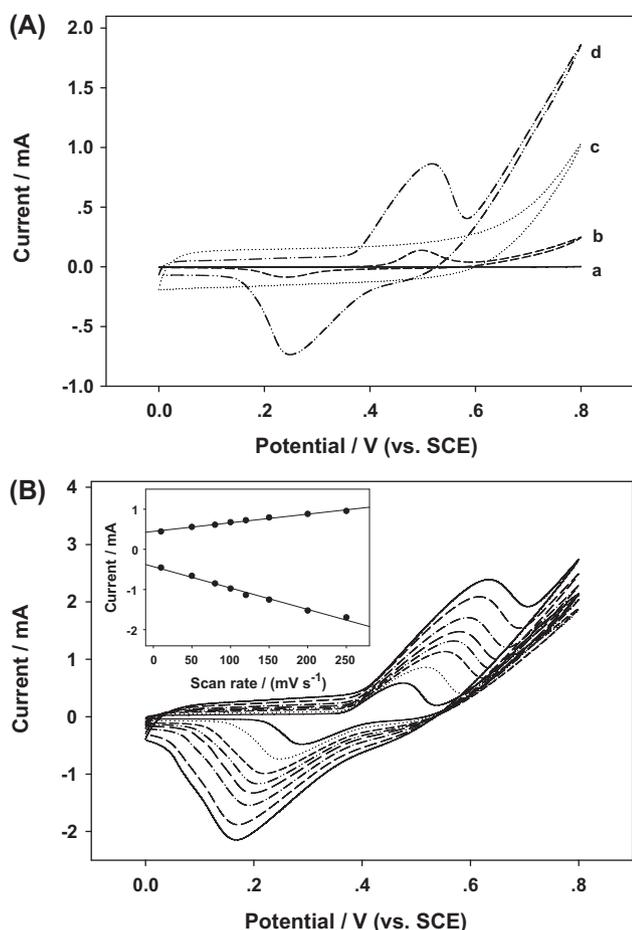
**Fig. 2.** Cyclic voltammograms obtained in 0.1 M NaOH solution at bare (a), NiNPs (b), SMWNTs (c) and NiNPs/SMWNTs nano hybrids (d).
