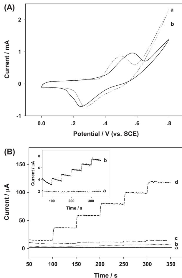
**Fig. 3.** Cyclic voltammograms of the NiNPs/SMWNTs modified electrode in 0.1 M NaOH solution with (curve b) and without (curve a) 2 mM glucose at a scan rate of 50  $\text{mV s}^{-1}$  (A) and amperometric responses of bare (a), NiNPs (b), SMWNTs (c), and NiNPs/SMWNTs (d) modified GC electrodes to successive addition of 100  $\mu\text{M}$  glucose in 0.1 M NaOH at +0.4 V (B).
